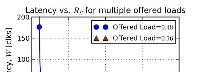
Offered load is the ratio of aggregate arrival rate to the peak service rate of the system and is equal to  $N \cdot \lambda \cdot t_{CLK}$ .
